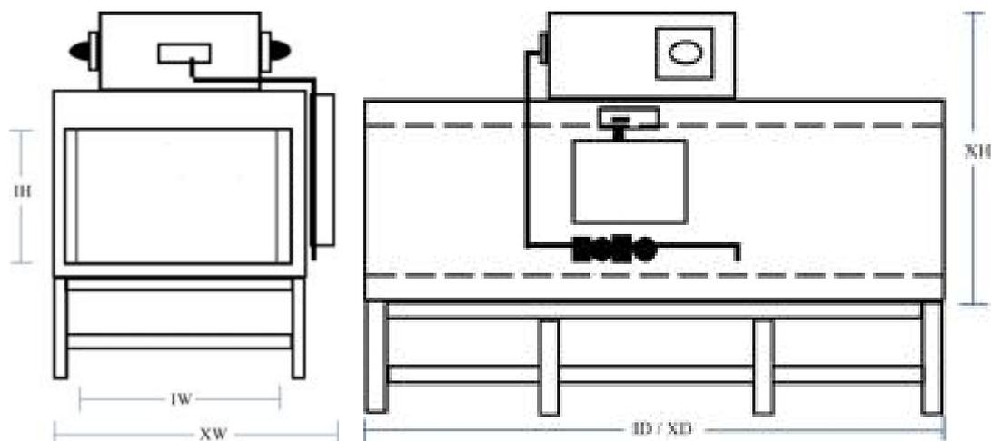
Profile of microwave baking and roasting equipment:
